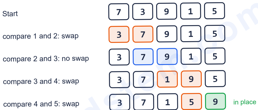
Fig. 1: in the first pass the largest value, 9, bubbles along to the end of the list
